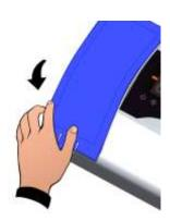
**Fig. 4:** Open the front panel of the box by lifting it and sliding the two hinges until they reach the end stop.
