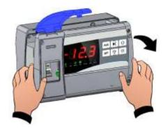
**Fig. 5:** Press on the sides of each hinge to unlodge it and completely remove the front panel.
