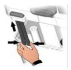
Fig. 6: Use the three pre-existing holes to fasten the base of the box with three adequately long screws based on the thickness of the wall that the panel will be installed on. Place a rubber washer (included) between each fastening screw and the base of the box.
